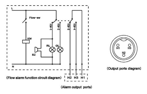
(2) Flow alarm causes of circulating cooling water and working state
